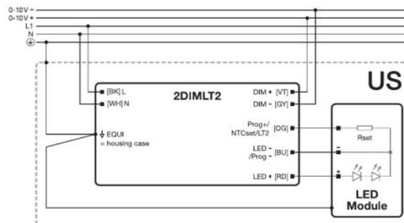
494749\_Wiring Diagramm 2DIMLT2 with LEDset2
