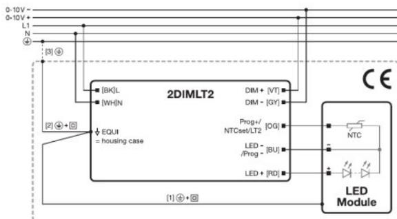
494748\_Wiring Diagramm 2DIMLT2 with NTC
